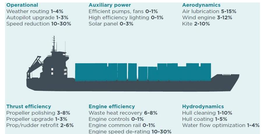
Figure 1: Potential fuel use and CO<sub>2</sub> reductions from various efficiency approaches for ships (International Council on Clean Transportation (ICCT), July 2013). Long-term potential for increased shipping efficiency through the adoption of industry-leading practices.
