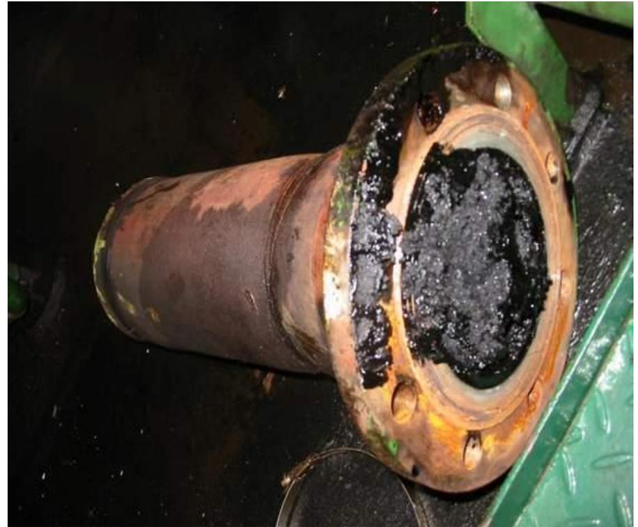
Clogged fuel pipes due to poor quality of fuel
