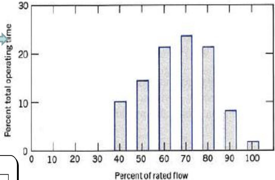
Load profile for a typical pump.
